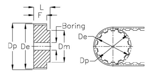
Belt width Type = T5= - 10 mm Weight = 0.307= 75.55 De Dm = 50 = 76.55 Dp F = 15 L = 21 Pre-drilled = 8
